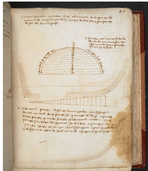
Byzantine whole-moulding methods from The Notebook of Zorzi Trombetta from Modon (1444-1449). British Library, Cotton Ms Titus A XXVI, fol. 45r
